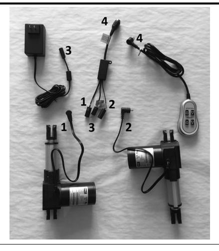
Remove and discard the movement remote and control box.
